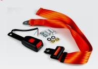
Length up to 120cm including buckle. Buckle on metal strap 10cm. 2"/47mm wide. Micro switch for wearing check/vehicle immobilisation capability. Switch rating: 12 volt=2amp. 24 volt=1amp. 45 volt=0.5amp. Comes with all fixings.
